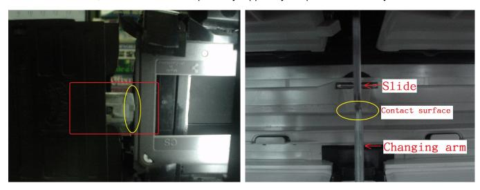
If the arm is not aligning in the center, you must gently press the Tappet arm in the opposite direction of the mis-alignment
