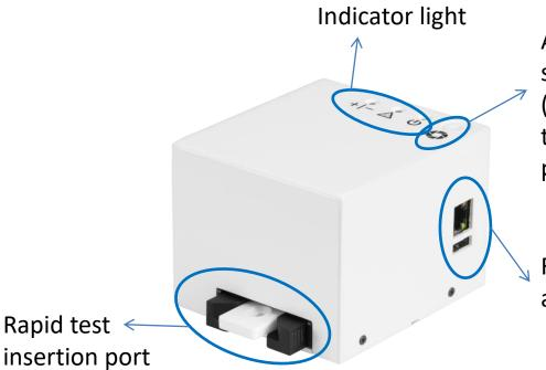
Analysis button, switch button (Short press to turn on, long press to turn off)
